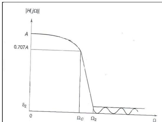
Figure 4: Magnitude response of a low pass Chebyshev Type II filter
