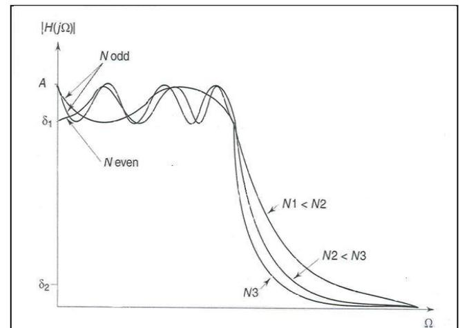
**Figure 3:** Magnitude response of a low pass Chebyshev Type I filter.
