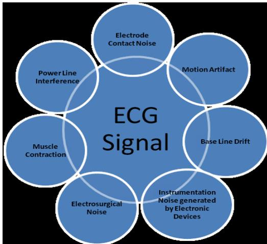
**Figure 2:** Interferences in the ECG signal.
