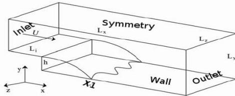
**Figure 1:** Computational domain and boundary conditions
