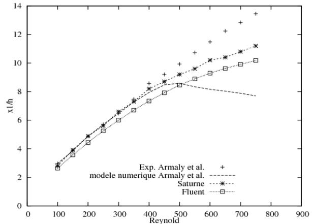
**Figure 2:** Comparison of experimental and numerical measurements for the reattachment length for  $Re < 800$
