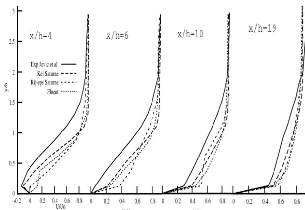
**Figure 3:** Normalized mean stream wise velocities ( $U/U_0$ ) at the locations  $x/h=4, 6, 10$  and  $19$
