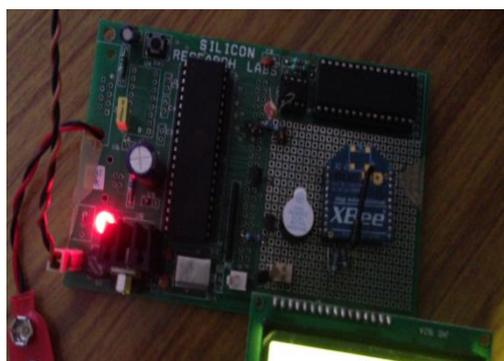
Figure 4: Sensor board.
