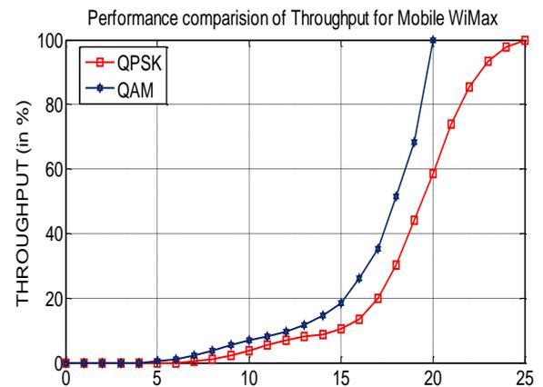
**Figure 5:** Performance of IEEE 802.16e MAC Layer over AWGN Channel with comparison Modulation Techniques of QPSK and QAM
