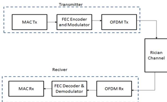
**Figure 1:** Block diagram of WiMAX Simulation Model
