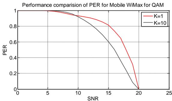
**Figure 2:** Performance of IEEE 802.16e MAC Layer over AWGN with QPSK Modulation Scheme
