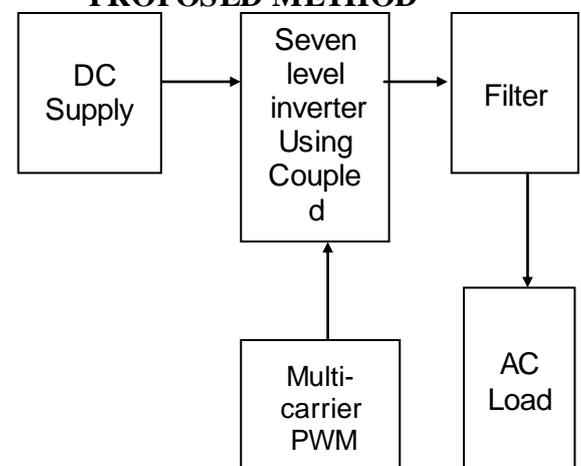
Figure 1: Block Diagram
