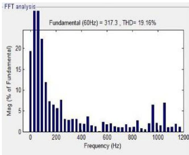
Figure 5: FFT Analysis for Seven Level Inverter
