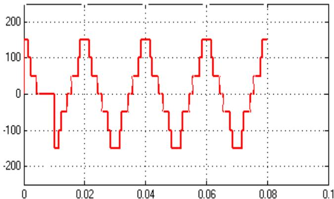
Figure 4. Output Voltage for Seven Level Inverter
