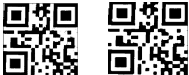
Figure 7: Comparison QR-Code without/with Median filter
