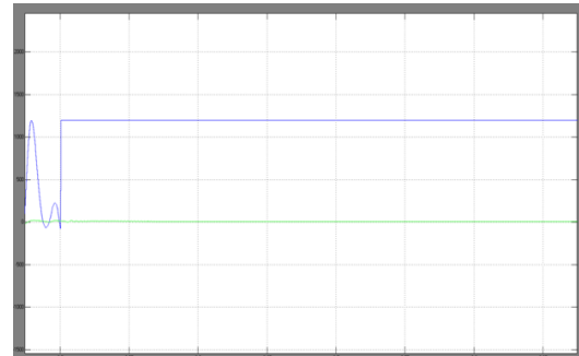
Figure 10: Comparison of simulation results of the DTC of IMD using both Electromagnetic Torque developed and reference torque given to the Torque control IM
