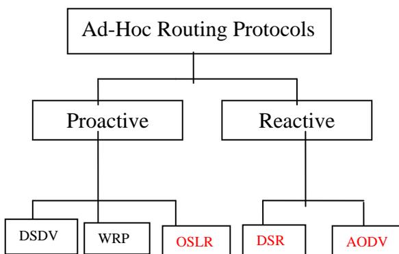
**Figure 3:** Classification of routing protocols
