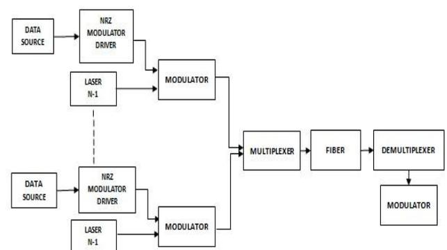
**Figure1** Schematic model for NRZ
