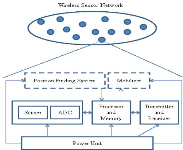
Figure 1. WSN and components of sensor node
