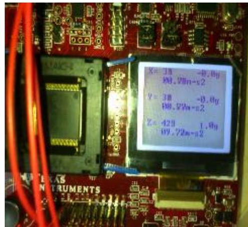
Figure 5: Acceleration 'g' values displayed on GLCD
