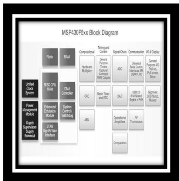
**Figure2:** Block diagram of the MSP430F5438A Microcontroller
