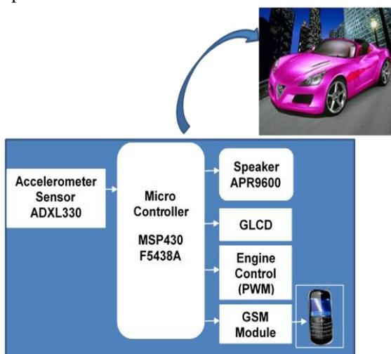
**Figure1:** Hardware Architecture of the monitoring system.
