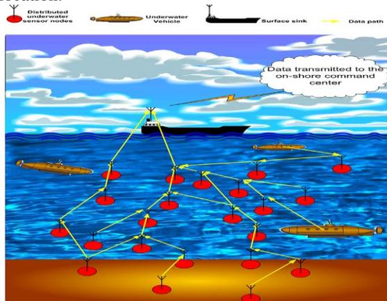
**Figure 1:** Underwater wireless sensor networks (UWSNs). [1]
