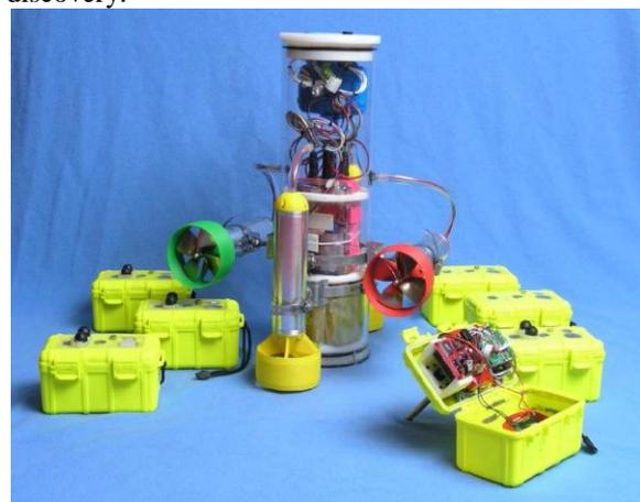
**Figure 2:** Group photo of the underwater sensor nodes. (a) the static sensor nodes (Aquaflecks) and a mobile node (Amour AUV) [4].
