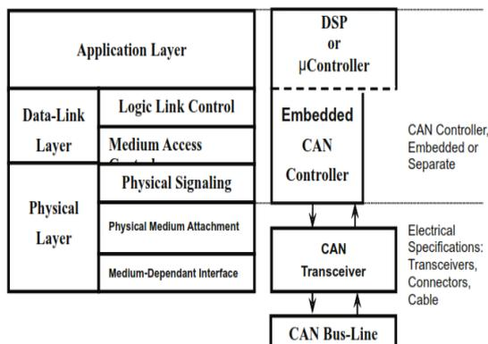
Figure 1: The Layered ISO 11898 Standard Architecture
