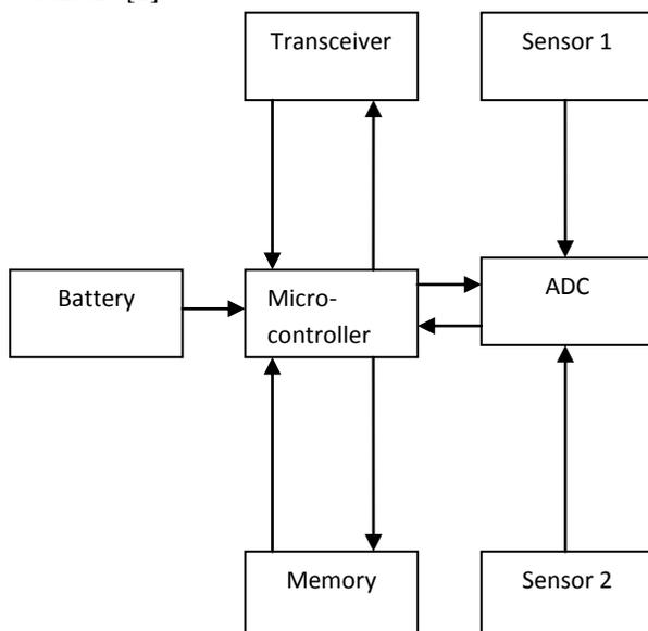
Figure 1: A typical architecture of the sensor node [1]
