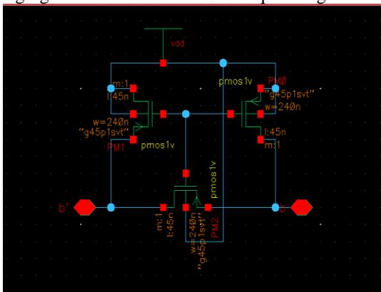
**Figure 3:** Pre Charge Circuit
