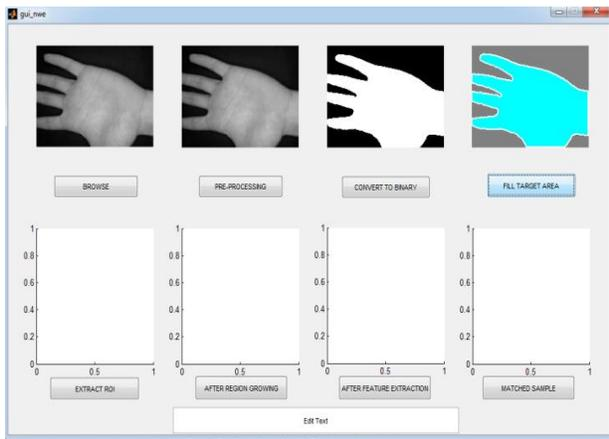
**Figure 5:** This graph represents the second step of ROI extraction in which image is filled with the color before extracting sub-image
