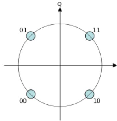
**Figure 4:** Constellation diagram for QPSK with Gray coding.
