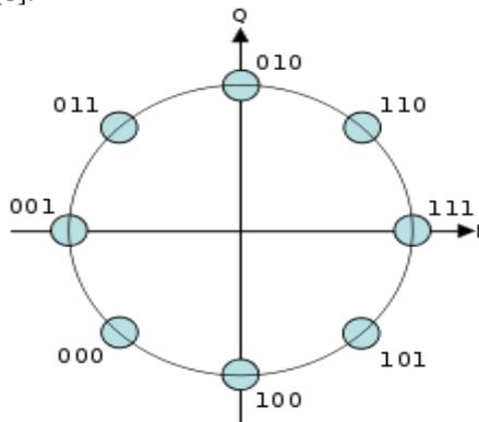
**Figure 3:** A constellation diagram for Gray encoded 8-PSK.
