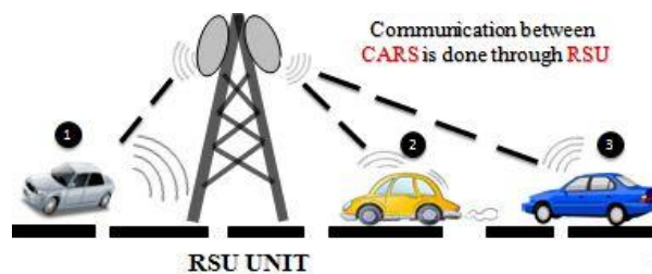
Figure 2: Vehicle to roadside communication
