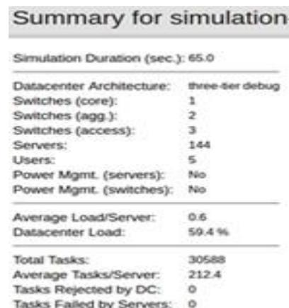
Figure 1.3: Output after executing the Round Robin Scheduling Algorithm using VM under Linear power model
