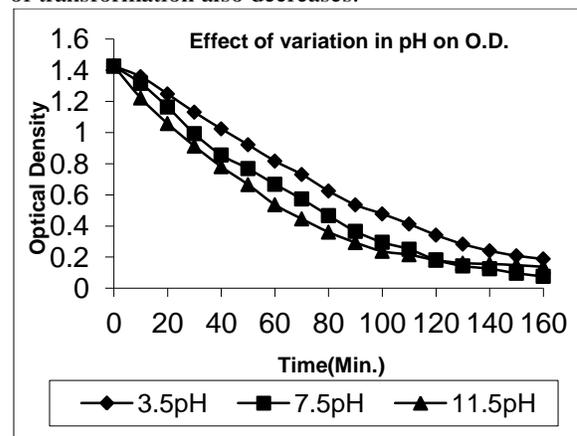
**Fig-5:** Effect of pH on transformation (Temperature: 303 K, solution volume: 50 ml, initial dye concentration: 40 mg/l, UV lamp: 10.4 mW cm<sup>-2</sup>.)
