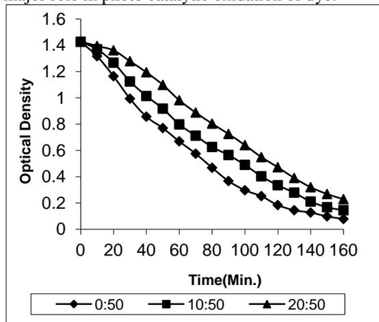
**Fig-7:** Effect of variation of quencher on transformation (Temperature: 303 K, solution volume: 50 ml, initial dye concentration: 40 mg/l, pH 7.5.)
