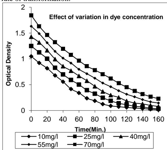
**Fig-4:** Effect of initial dye concentration on transformation (Temperature: 303 K, solution volume: 50 ml, pH 7.5, UV/visible lamp: 10.4 mWcm<sup>-2</sup>.)
