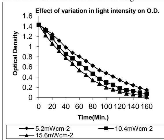
**Fig-6:** Effect of variation of light intensity on transformation (Temperature: 303 K, solution volume: 50 ml, initial dye concentration: 40 mg/l, pH 7.5.)
