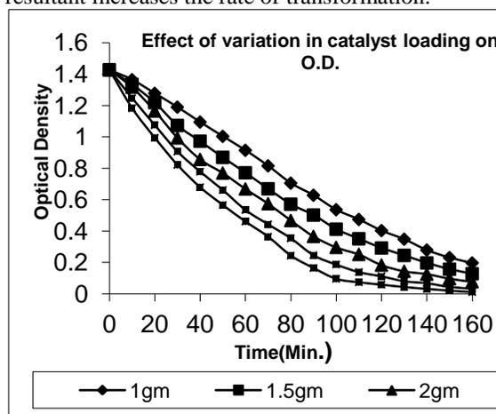
Fig-3: Effect of catalyst loading on photo catalytic transformation (Temperature: 303 K, solution volume: 50 ml, initial dye concentration: 40 mg/l, pH 7.5, UV /visible lamp: 10.4 mWcm<sup>-2</sup>.)
