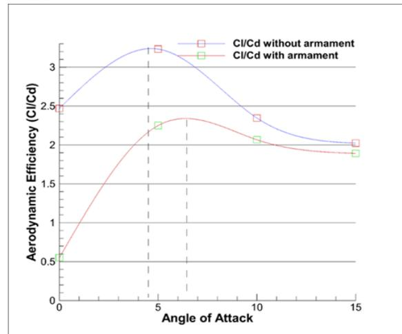
Figure 8: Aerodynamic efficiency vs. AOA
