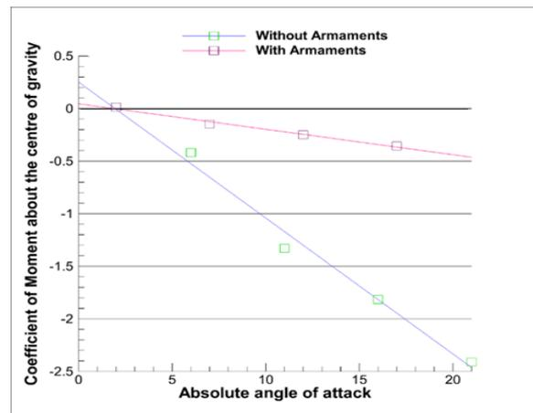
Figure 9: C<sub>M,cg</sub> vs. AOA for both configurations
