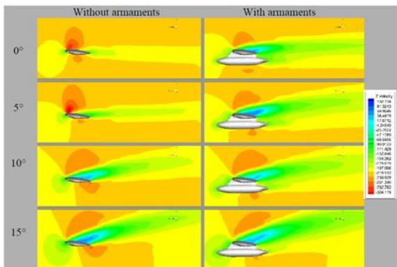
Figure 11: Velocity contours around the armament position
