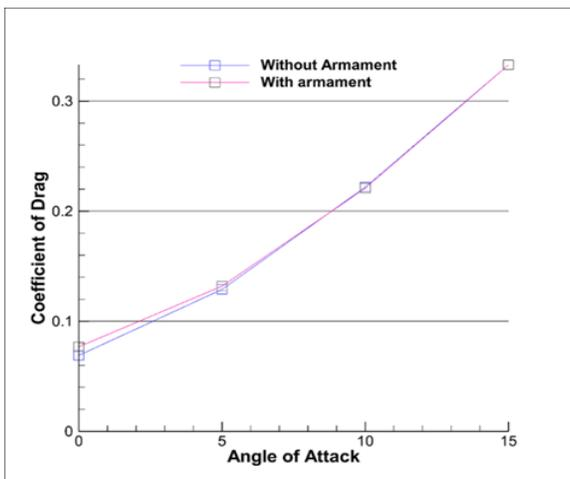
Figure 6: C<sub>D</sub> vs. AOA curves of both configurations
