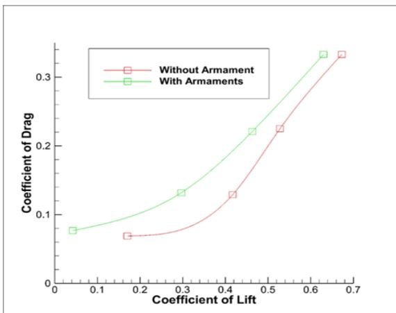
Figure 7: Drag polar curves of both configurations
