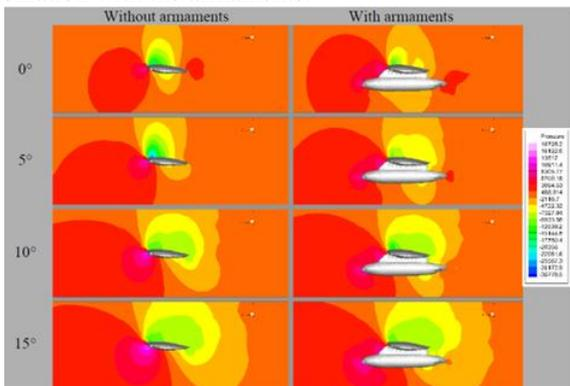
Figure 10: Pressure contours around the armament position
