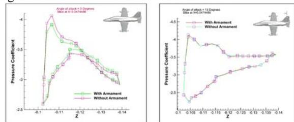
Figure 12:  $C_p$  curves at the centre of the wing for 0° and 15° AOA
