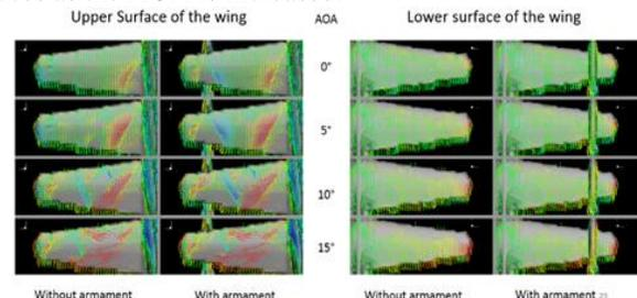
Figure 13: Velocity vectors coloured by the magnitude of spanwise flow
