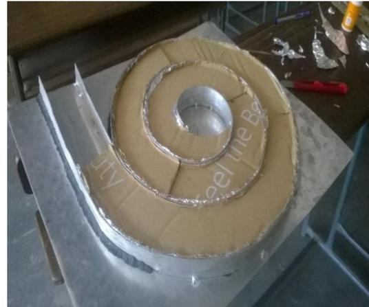
**Figure 4:** Vortex type absorber plate
