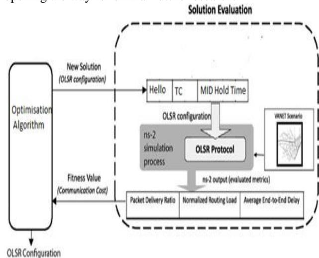
Figure 3: Optimization framework for automatic OLSR configuration
