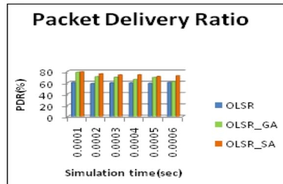
**Figure 4:** Comparison of Packet Delivery Ratio among OLSR, OLSR-GA and OLSR-SA
