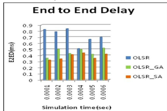
**Figure 5:** Comparison of End to End delay among OLSR, OLSR-GA and OLSR-SA
