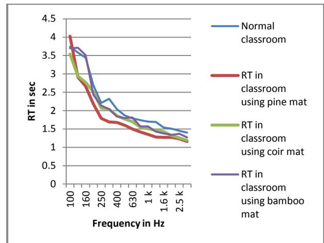
**Fig 6:** Averaged reverberation time in classroom before and after installing different absorbing panels.
