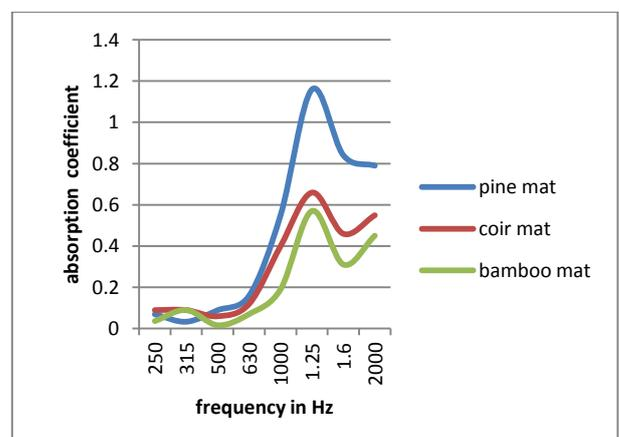
**Fig 8:** Sound absorption coefficient at different frequencies for pine mat, coir mat, and bamboo mat.
