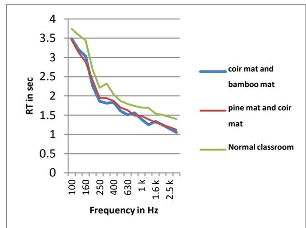
**Fig 7:** Reverberation time in classroom before and after installing combination of bamboo and pine mat panels, with coir mats on floor.
