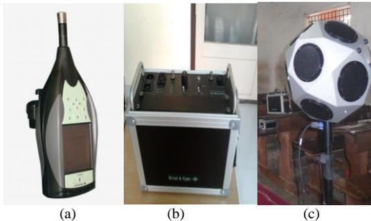
**Fig 3:** (a) Bruel and kjaer (BK 2250) sound level meter used for measuring Reverberation time. (b) 2734-B power amplifier. (c) 4292-L Omni Power sound source.
