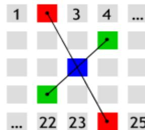
Figure 2: Symmetric Opposite Pixel pairs in SNN Filter
