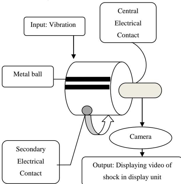
**Figure 7:** Block diagram of Car Camera Shock Sensor Cylinder.
