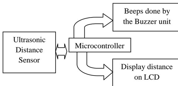
Figure 6: Block diagram of Algorithmic Move Car System
