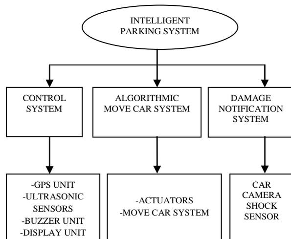
**Figure 1:** Block diagram of the proposed Intelligent Parking System
