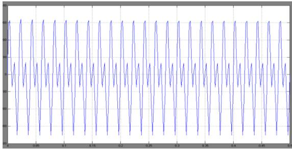
Fig -3(b): Input Voltage before EMI filter
