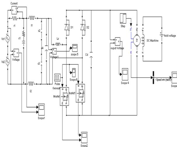
Fig -4(a): Simulation circuit of open loop system
