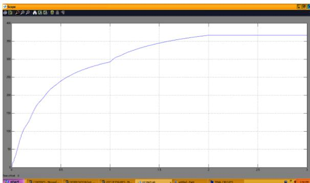
Fig -4(b): Rotor speed (Rad/Sec) with disturbance in open loop system
