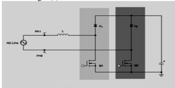
**Fig -1:** Bridgeless PFC circuit
