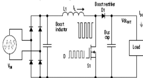
**Fig -1(a):** Conventional PFC circuit
