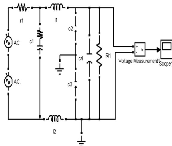
**Fig -3(a):** EMI filter circuit
