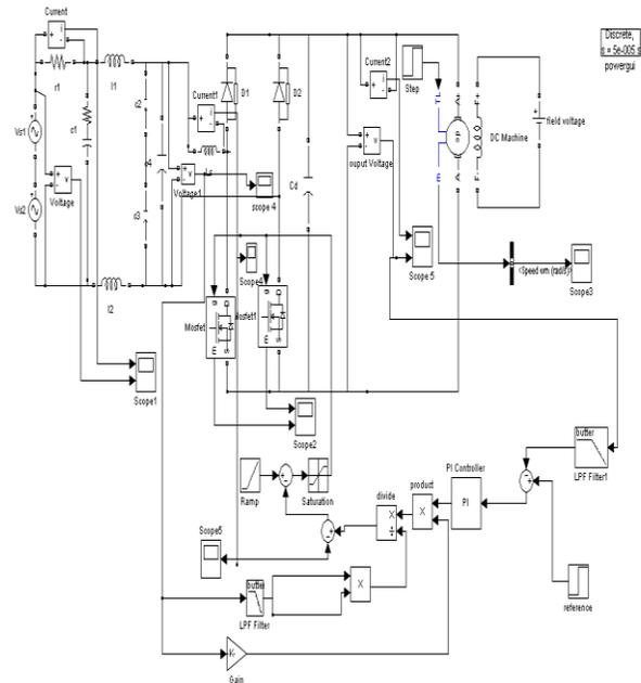
Fig -5(a): Circuit diagram for closed loop system
