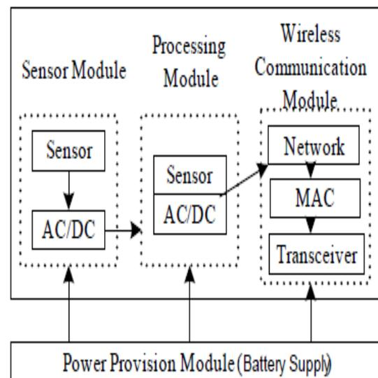
**Fig 1.1:** The architecture of a WSN Node Network.
