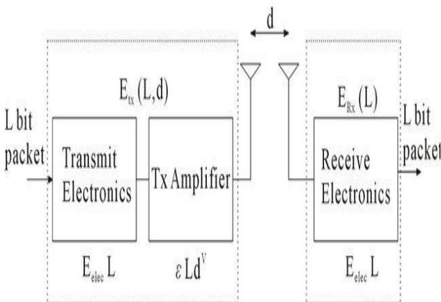
**Fig 1.5:** Radio Energy Dissipation Model
