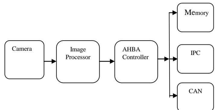
**Figure 1:** Block Diagram of AHBA
