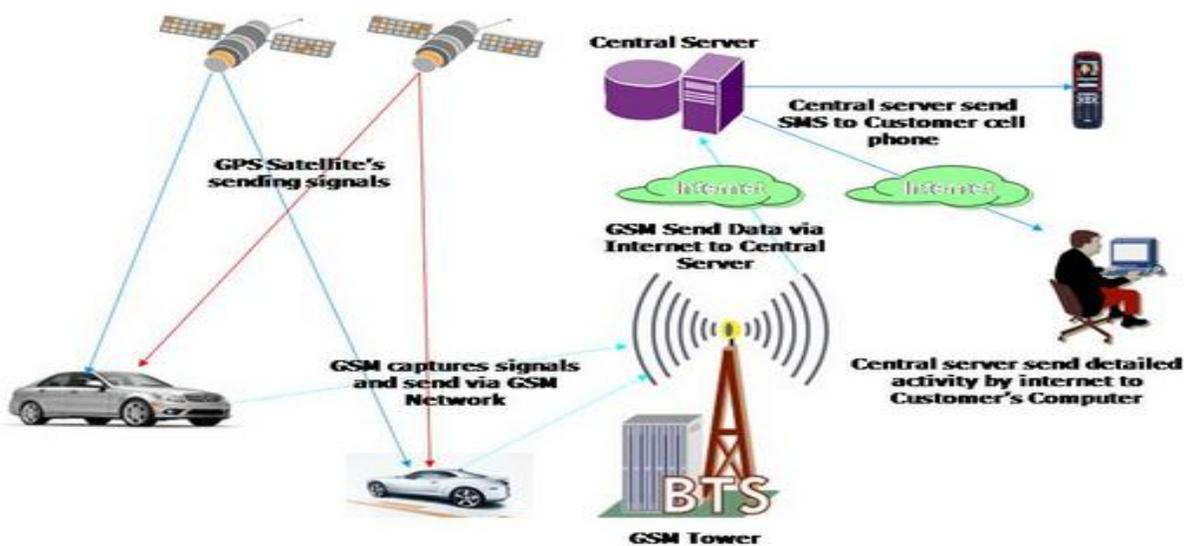
Figure1: vehicle tracking system
