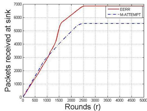
**Figure 6:** No. of Rounds vs Data received at Base Station (SINK)
