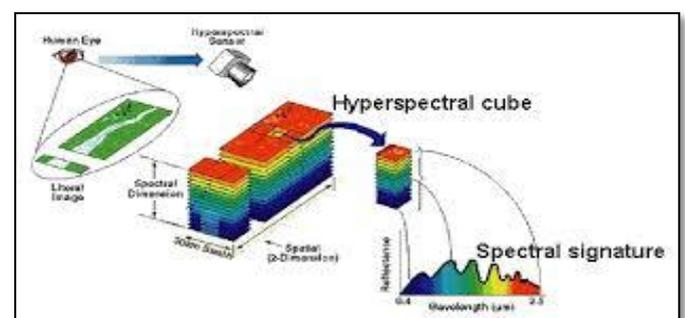
Figure 1: Hyperspectral Imaging
