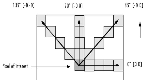
Figure 5: Multiple orientations to calculate GLCM
