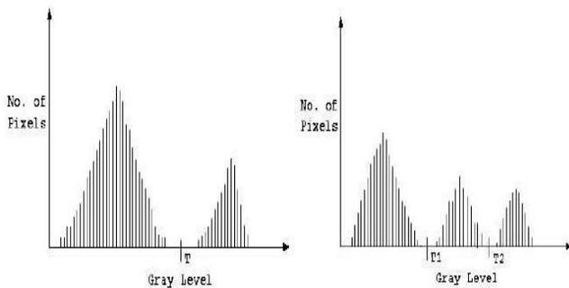
**Figure 2:** Gray-level histograms that can be partitioned by (a) a single threshold, and (b) multiple thresholds
