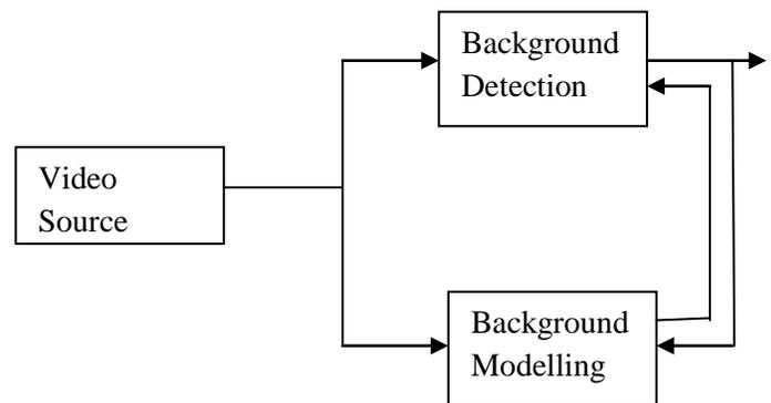
**Figure 1:** A video source produces images I. The modeling stage uses previous video frames and detection results to maintain background model B. The detection stage compares the current frame to the current model to produce a detection mask E.
