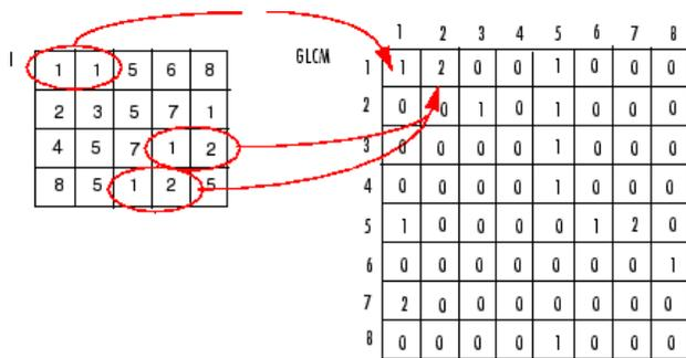
Figure 4: GLCM output of a test matrix.
