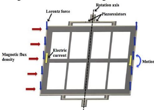
Figure 3: Operation Principle of a MEMS Magnetic Field Sensor
