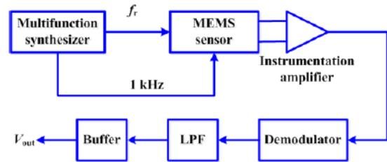
Figure 4: Signal Conditioning Stages Of The MEMS Magnetic Field Sensor
