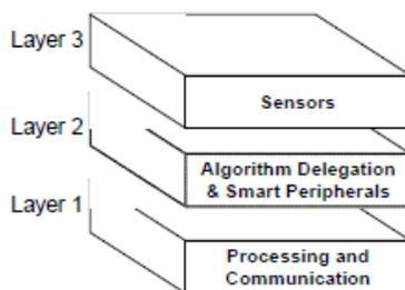
**Figure 7:** Sensor node hardware stack
