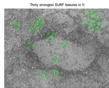
Figure 5: SURF feature extraction of left image
