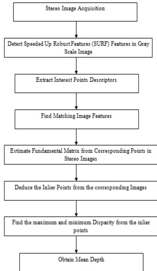
**Figure 2:** Stereo vision Un-calibrated rectification Process
