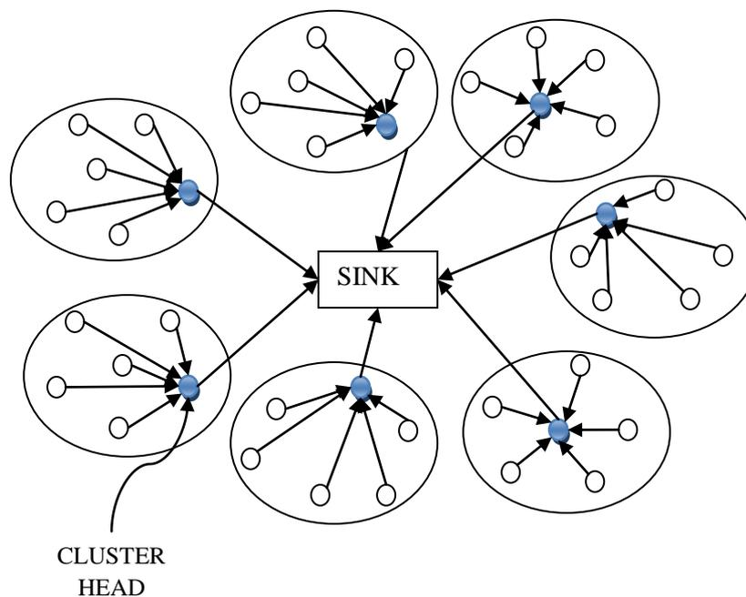
**Figure 3:** Clustering Schema for Wireless Sensor Networks [5]
