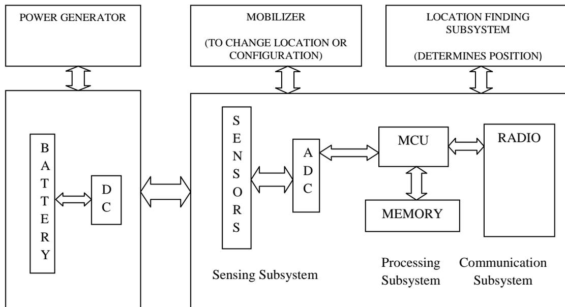
Figure 2: Architecture of a Sensor Node [4]
