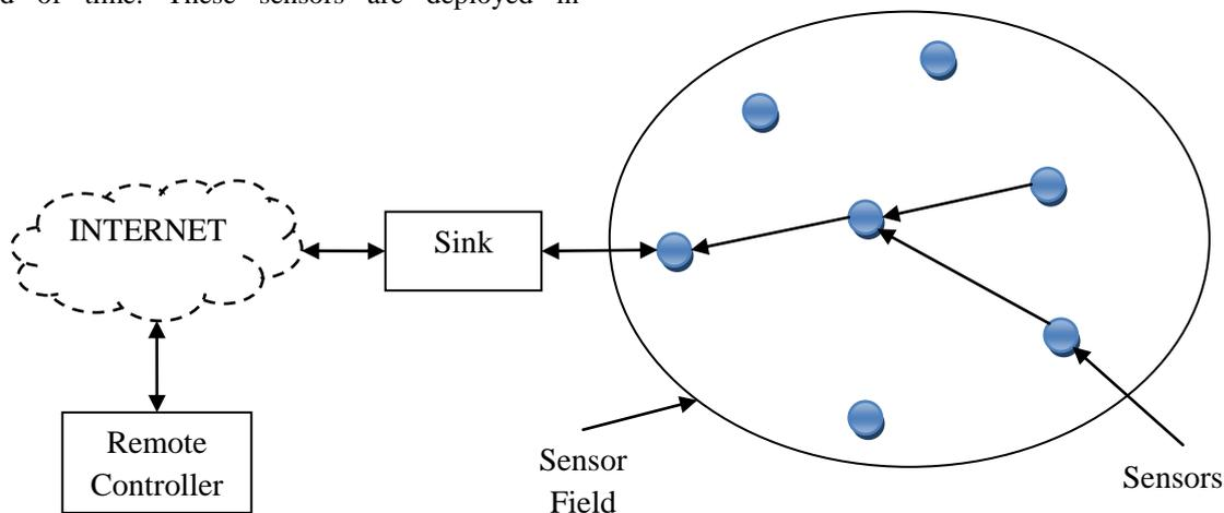
**Figure 1:** Architecture of Wireless Sensor Networks [2]
