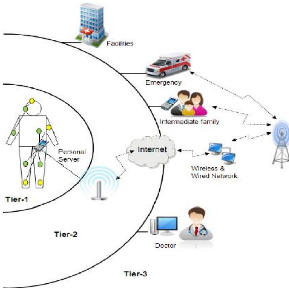
**Figure 1:** Communication Tiers in a Wireless Body Area Network [8]
