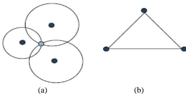
**Figure 1:** (a) Tri-Lateration & (b) Triangulation
