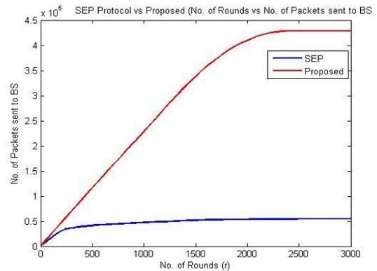
**Figure 5:** Number of Rounds vs Data Packets sent to base station (SINK)
