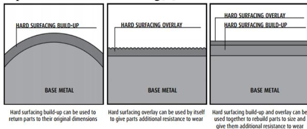
Figure 1.1: Hardfacing application
