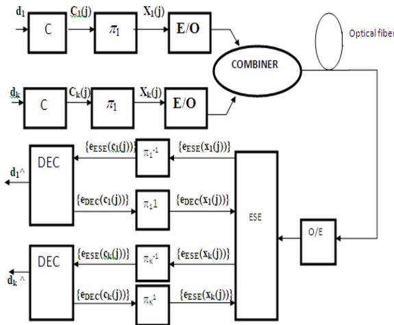
**Figure -1:** Optical IDMA Transmitter and Receiver Structure.
