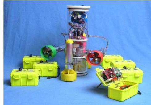
**Figure 2:** Group photo of the underwater sensor nodes.
