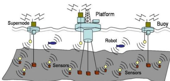
Figure 1: Underwater Sensor Network Architecture [6]
