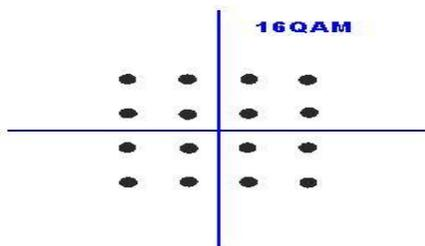
**Figure 4:** Constellation Diagram of 16 – QAM [8]
