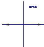
**Figure 2:** Constellation Diagram of BPSK [8]
