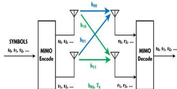
Figure 1: MIMO System (2X2 MIMO Channel)
