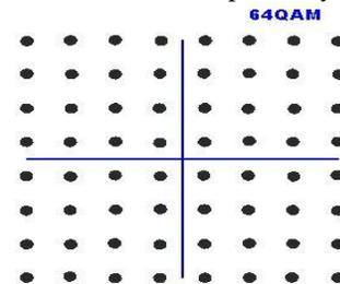
**Figure 6:** Constellation Diagram of 64 – QAM [8]
