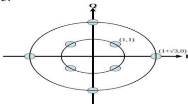
**Figure 3:** Constellation Diagram of 8 – QAM [8]
