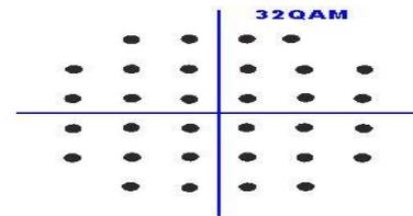
**Figure 5:** Constellation Diagram of 32 – QAM [8]
