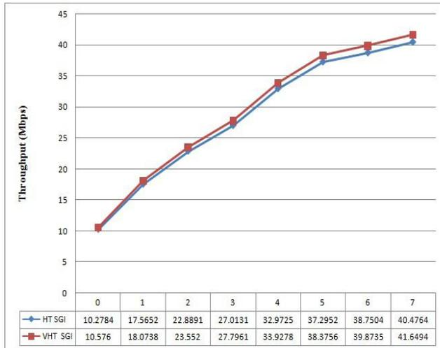
Figure 5: Throughput vs. MCS; Short GI and 40 MHz bandwidth.
