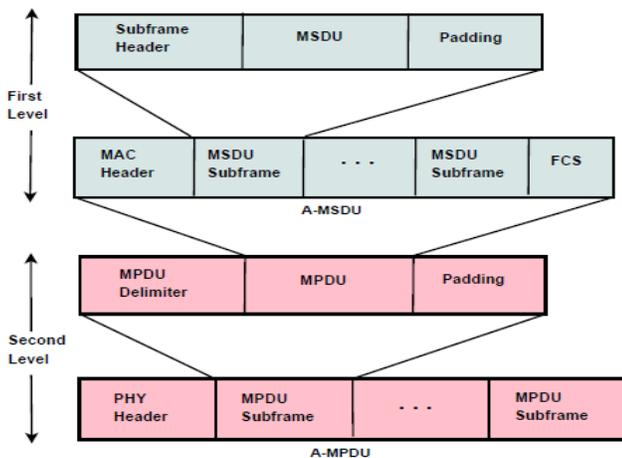
Figure 2: Two level frame aggregation
