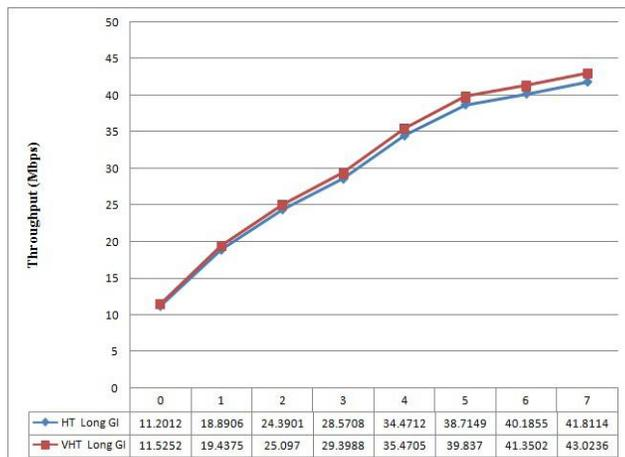
Figure 6: Throughput vs. MCS; Long GI and 40MHz.
