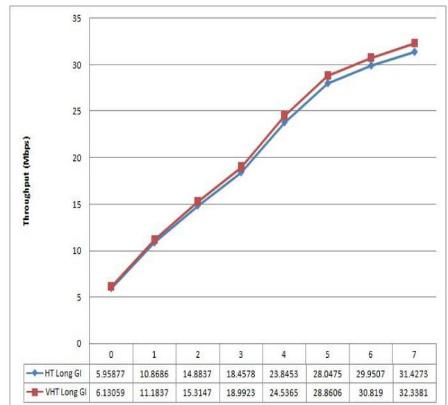
Figure 4: Throughput vs. MCS; Long GI 20 MHz bandwidth.
