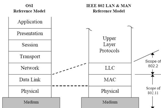
Figure 1: IEEE 802.11 standard and OSI reference model
