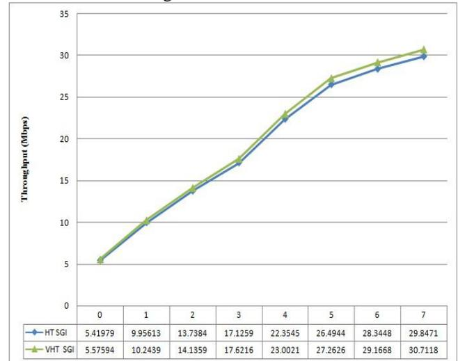
Figure 3: Throughput vs. MCS; Short GI and 20 MHz bandwidth.
