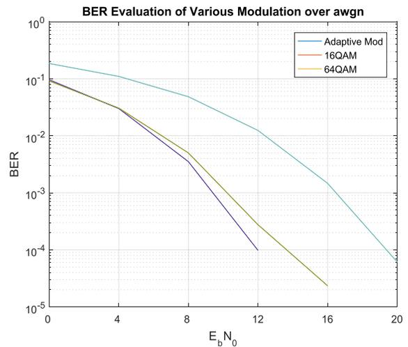
**Figure 3:** BER Evaluation of Adaptive Modulation, 16-QAM, 64-QAM over AWGN channel SNR = [0:4:30] Simulation Frames 1000, AMC outperforms all other modulation techniques
