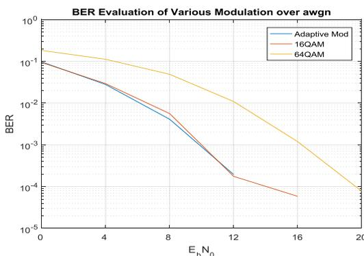
**Figure 2:** BER Evaluation of Adaptive Modulation, 16-QAM, 64-QAM over AWGN channel SNR = [0:4:30] Simulation Frames 100, AMC outperforms all other modulation techniques
