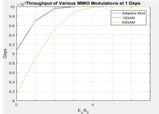
**Figure 4:** Throughput Evaluation of Adaptive Modulation, 16-QAM, 64-QAM over AWGN channel SNR = [0:4:30] Simulation Frames 1000, AMC outperforms all other modulation techniques
