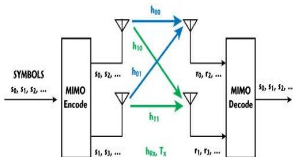
Figure 1: MIMO System (2X2 MIMO Channel)
