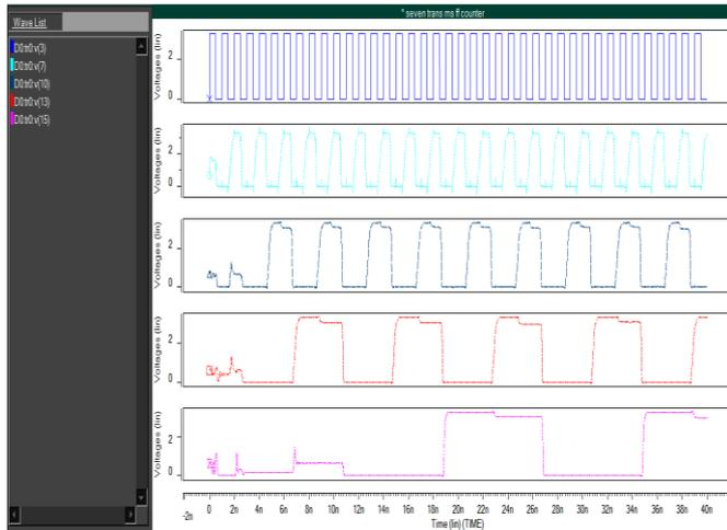
Figure 9: Output waveform of proposed down counter.
