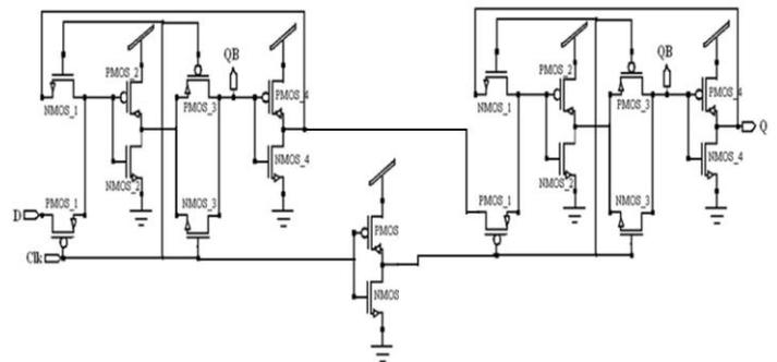
**Figure 3:** Flip flop using 8-Transistor latch.
