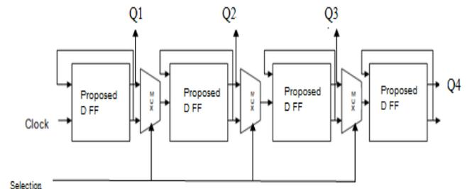
**Figure 8:** Up/Down counter using proposed D flip flop.
