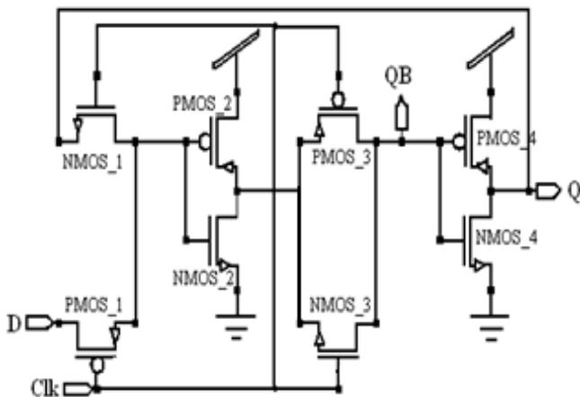
**Figure1:** 8-TransistorLatch Design.
