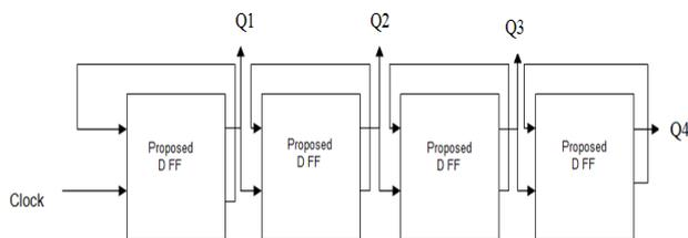
**Figure 5:** Up counter using proposed D flip-flop.
