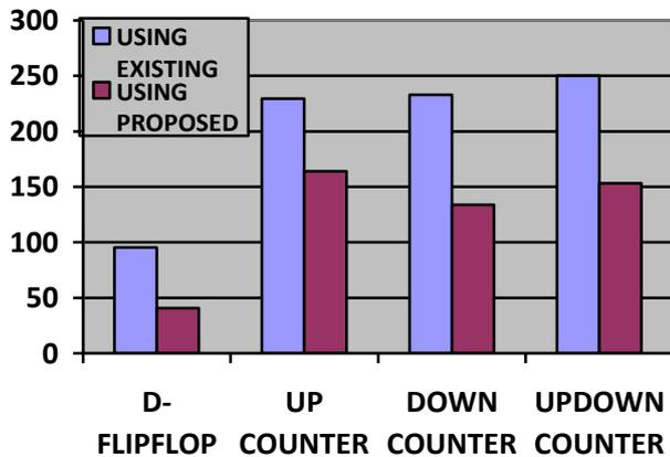
Figure 12: Power comparison graph of counters.
