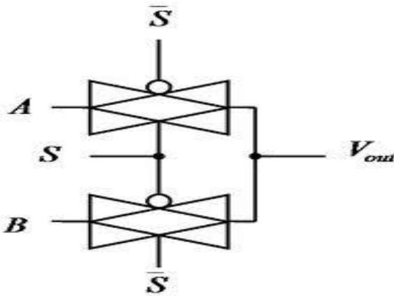
**Figure 5:** Transmission gate multiplexer.
