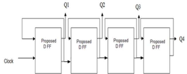
**Figure 7:** Down counter using the proposed D flip flop.
