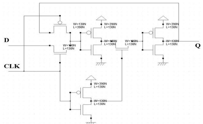
**Figure 4:** Proposed 9 transistors flip flop.
