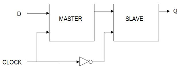
**Figure 2:** Master Slave flip flop.
