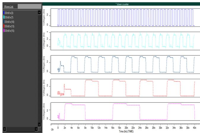
Figure 10: Output waveform of the proposed down counter.
