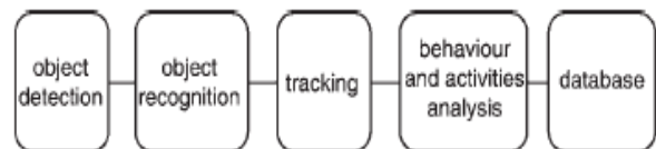
Fig. 1 Traditional flow of processing in visual surveillance system
