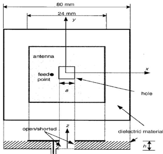
Fig. 1 Structure of the square patch with a square hole
