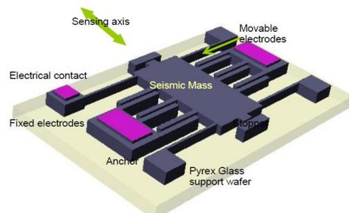
Fig. 1 Sensor Structure
