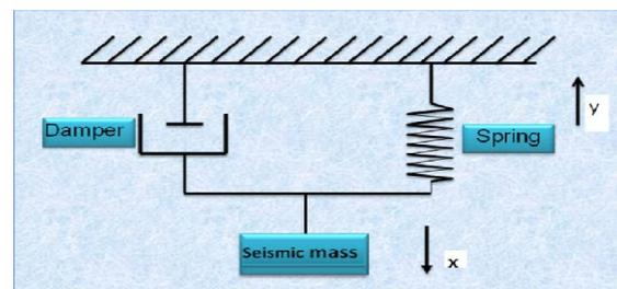
Fig.2 Mass Spring Damper system
