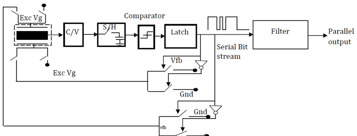
Fig. 4 signal conditioning circuit
