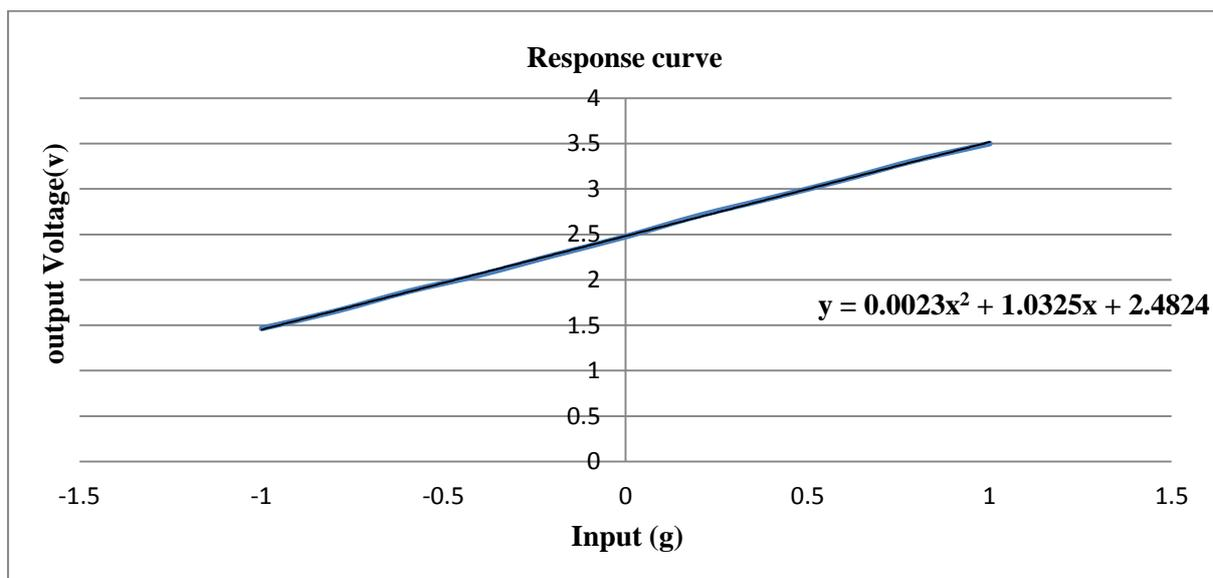
Fig. 6 Response curve ( Input g Vs Output Voltage)
